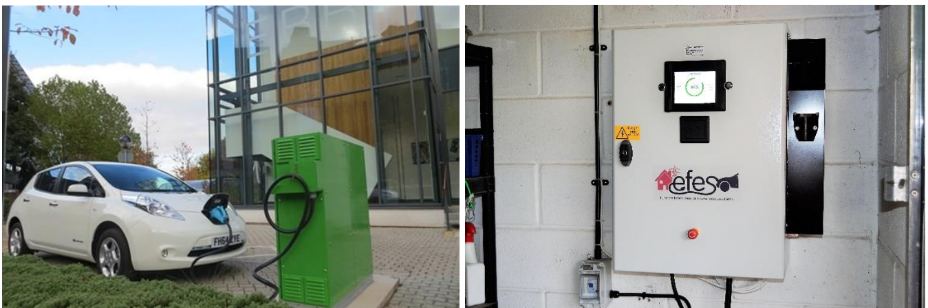
Figure 5: Early prototype V2G units in the UK - Commercial building (left) and domestic unit right)
