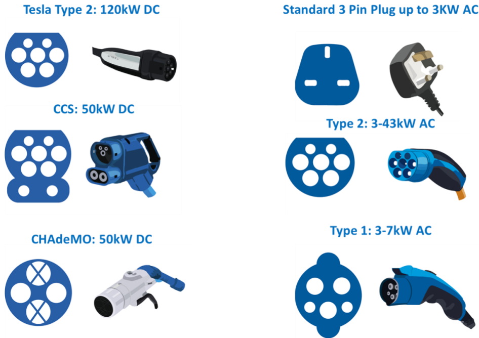
Figure 7 Types of Slow, Fast and Rapid Connectors
