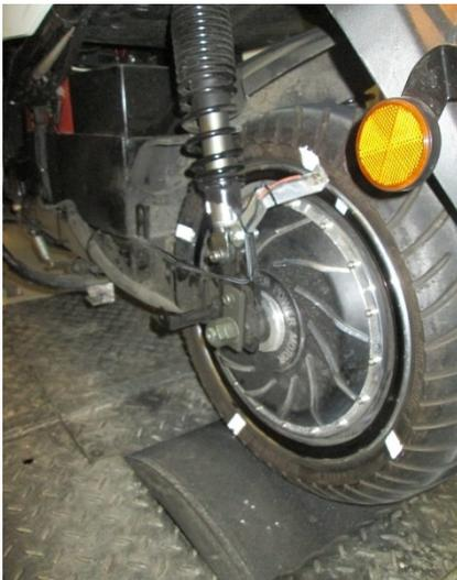
Figure 8: Rear tyre on dynamometer roller
