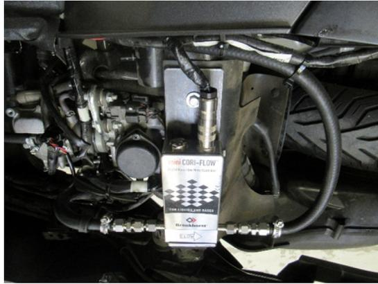
Figure 11: Fuel flow meter in petrol scooter
