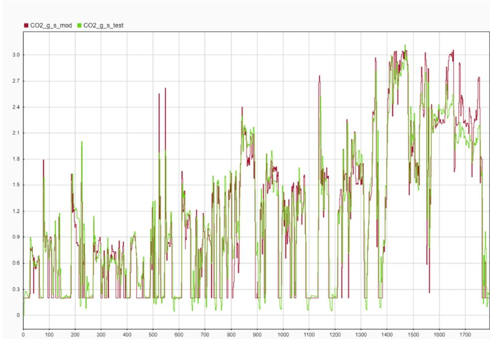
Figure 28: WMTC calibration of CO<sub>2</sub> emissions in grams per second
