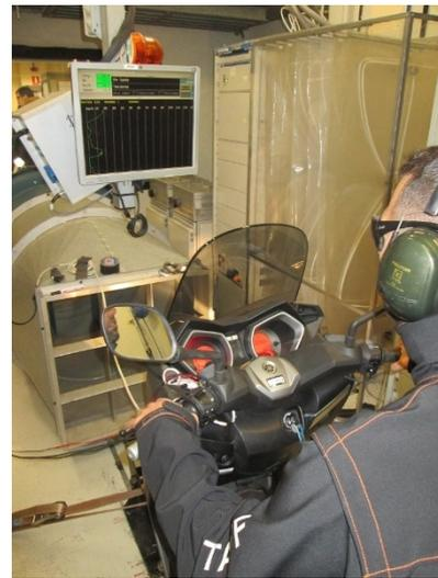
Figure 9: Dynamometer testing setup
