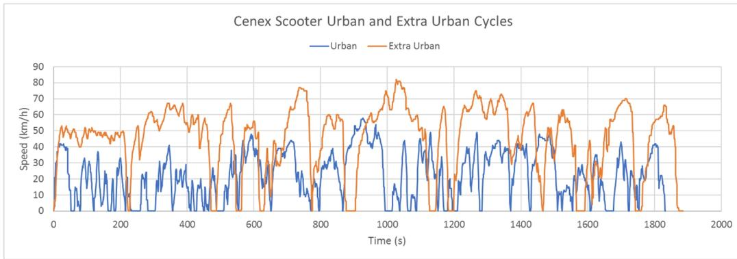
Figure 5: Representative scooter drive cycles generated by Cenex
