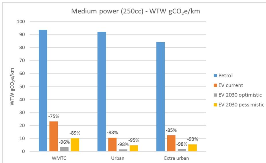
Figure 30: Simulated WTW GHG CO<sub>2</sub>e emissions for medium-power scooters
