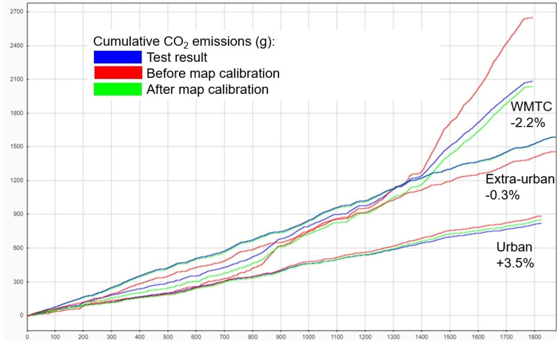
Figure 29: Calibration of cumulative CO<sub>2</sub> emissions
