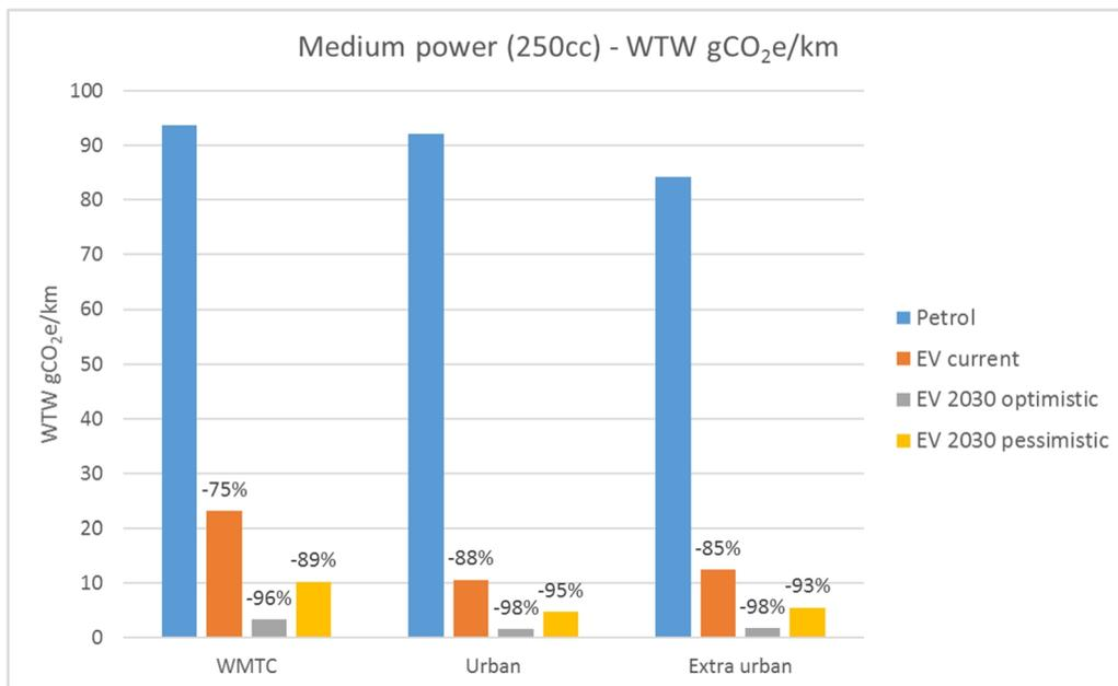
Figure 2: WTW CO<sub>2</sub>e emissions from simulation models
