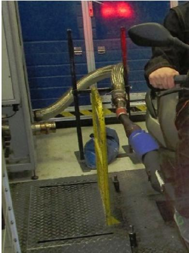
Figure 12: Tailpipe setup in the petrol scooter
