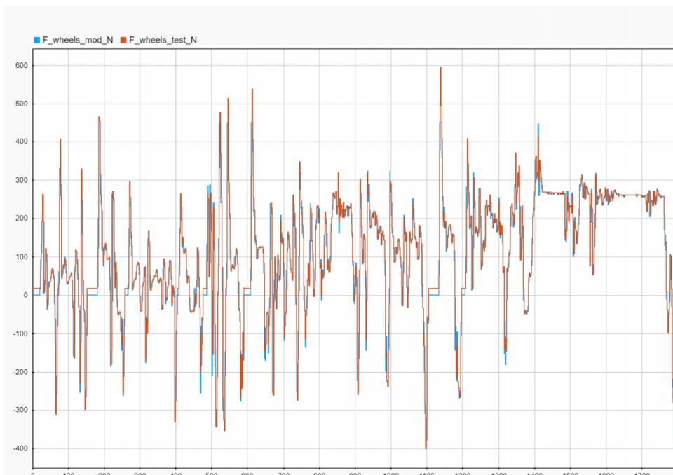
Figure 21: WMTc tractive force calibration in electric scooter
