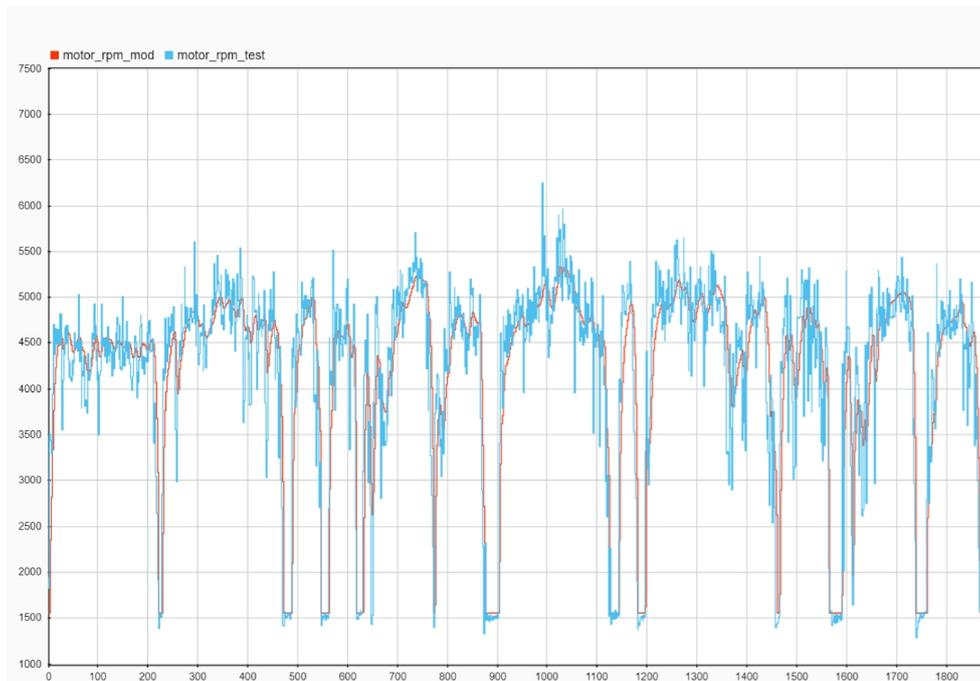
Figure 27: Extra urban calibration of motor rpm in petrol scooter
