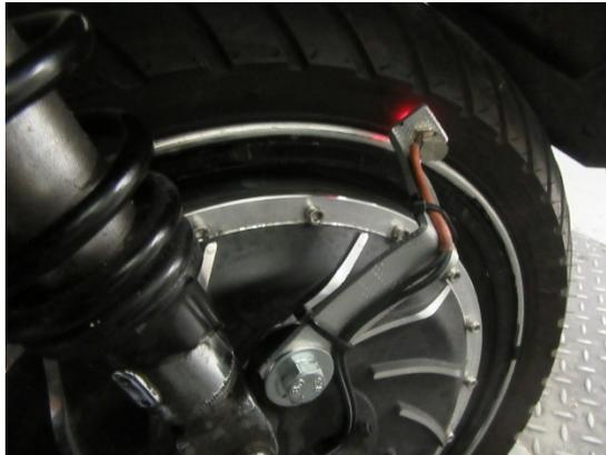
Figure 13: Tyre speed optical sensor
