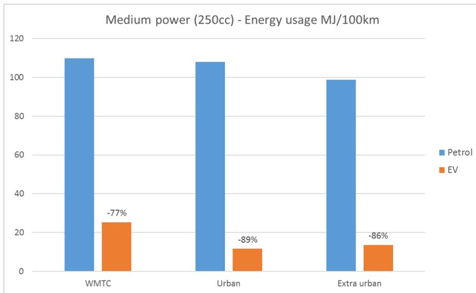
Figure 31: Simulated energy usage for medium-power scooters
