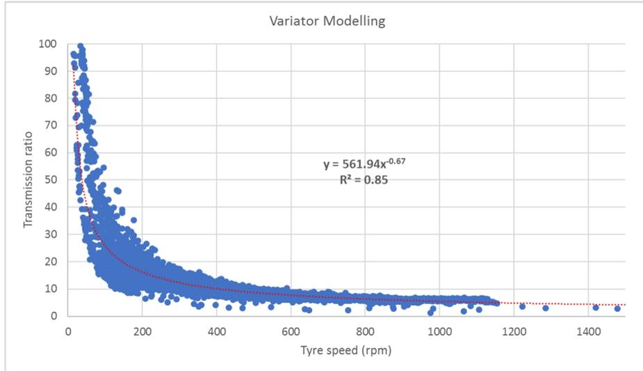
Figure 26: Power-curve fit of transmission ratio as a function of tyre speed
