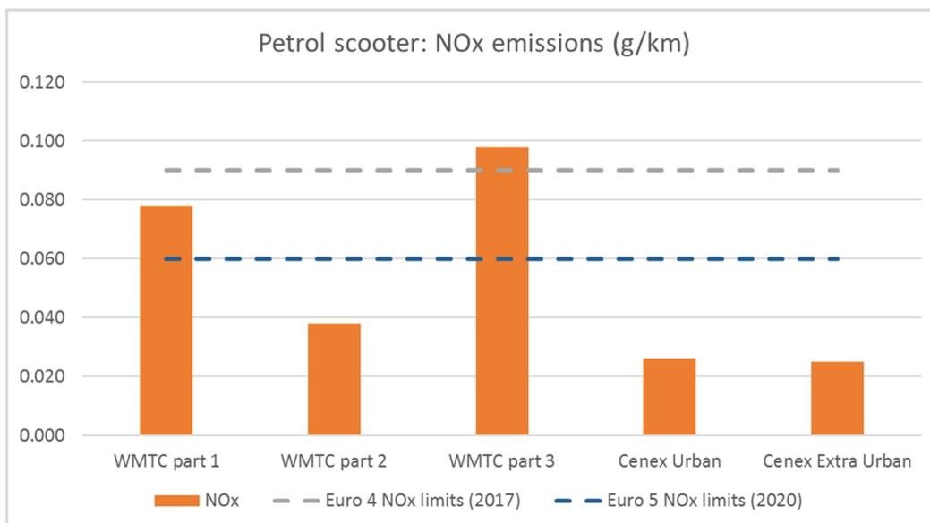
Figure 1: Tested NO<sub>x</sub> emissions vs regulatory limits
