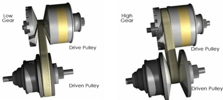
Figure 25: Different positions in a continuously variable transmission (CVT)
