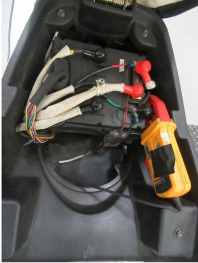
Figure 10: Current and voltage measuring equipment in electric scooter
