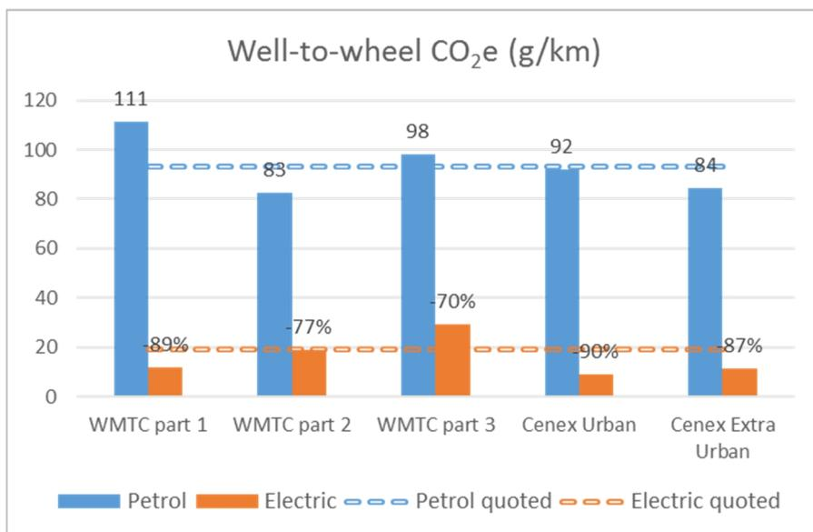
Figure 15: Test results - greenhouse gas WTW CO<sub>2</sub>e emissions
