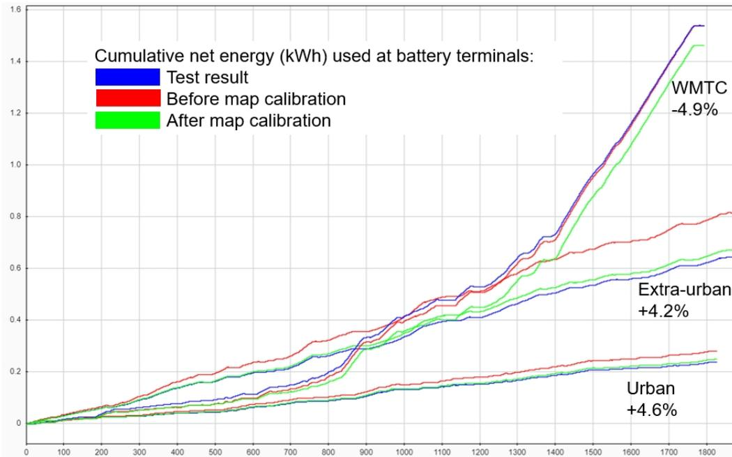
Figure 24: Calibration of cumulative net energy measured at battery terminals
