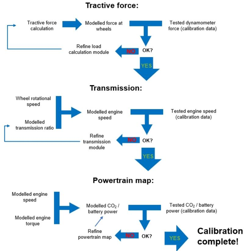
Figure 20: Process to calibrate a vehicle model
