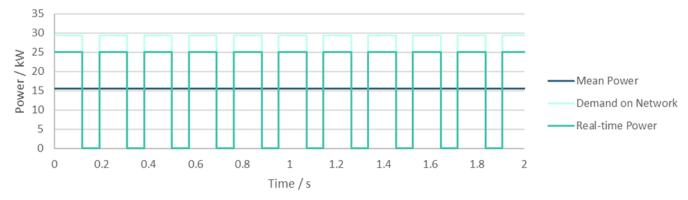
Figure 5-3: An Indicative Demand profile for a single vehicle, showing both the demand it would draw from the network, and the power delivered to the vehicle
