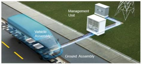
Figure 5-2: The layout of the ElectReon DWPT system
