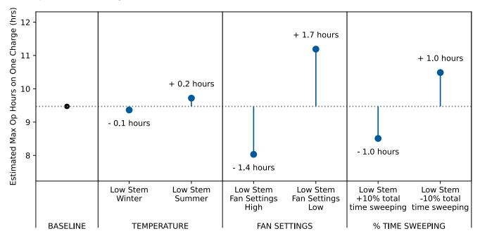
Figure 1: Estimated Impact of Duty Cycle Variations on Vehicle Operating Hours during a Low Stem Mileage Route.
