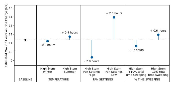
Figure 2: Estimated Impact of Duty Cycle Variations on Vehicle Operating Hours during a High Stem Mileage Route.
