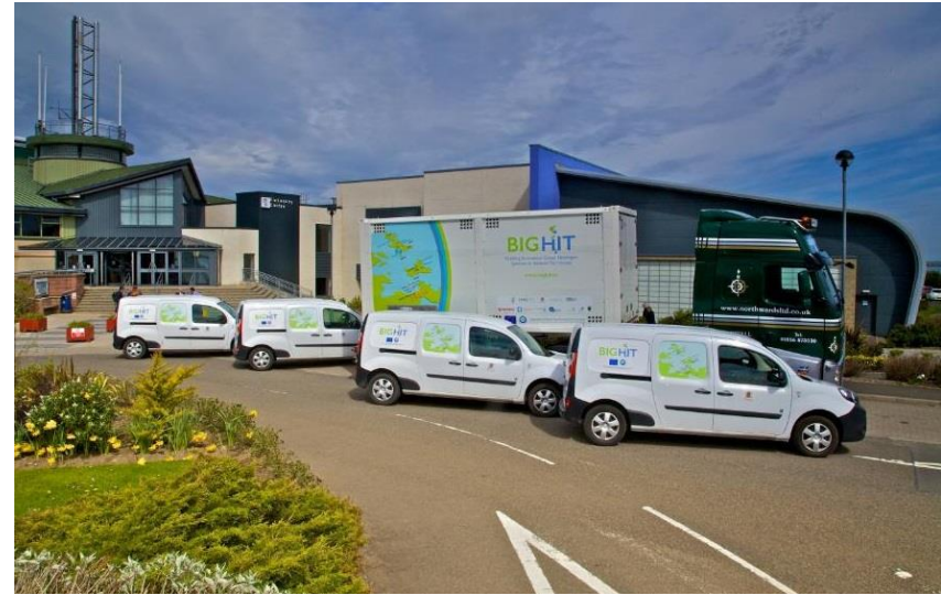
Hydrogen vans from Symbio used by Orkney Islands Council together with one of the five Calvera hydrogen trailers
