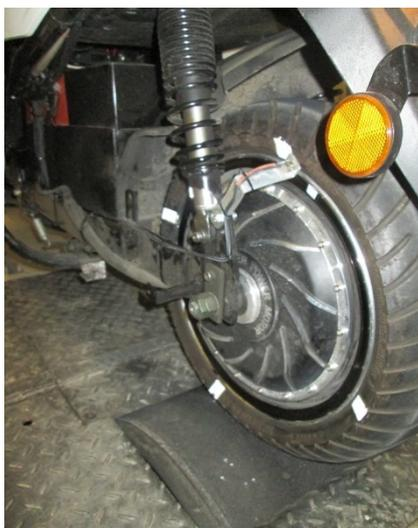
Figure 8: Rear tyre on dynamometer roller
