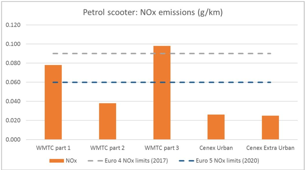
Figure 16: Comparison of NOx emissions with Euro limits
