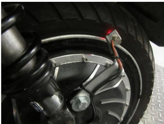
*Figure 13: Tyre speed optical sensor*
