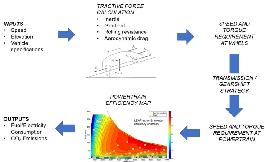
Figure 19: Vehicle model layout
