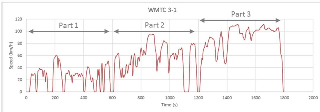
Figure 4: Legislative WMTC drive cycle (reduced speed version in part 3)
