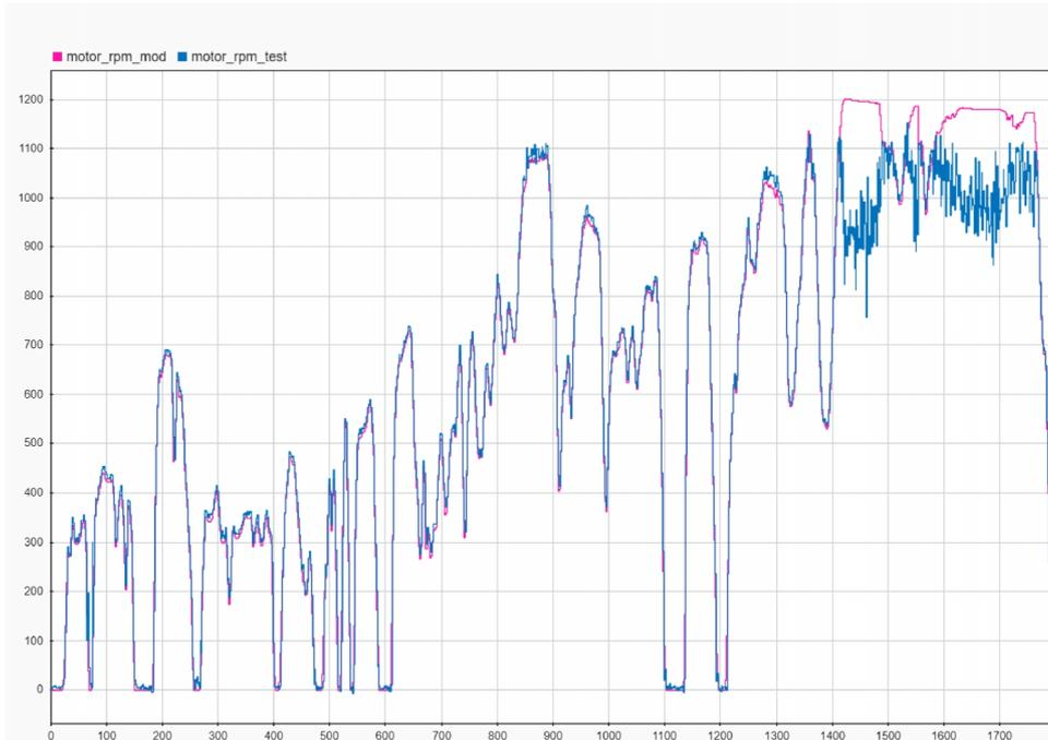
Figure 22: WMTC motor speed calibration in electric scooter
